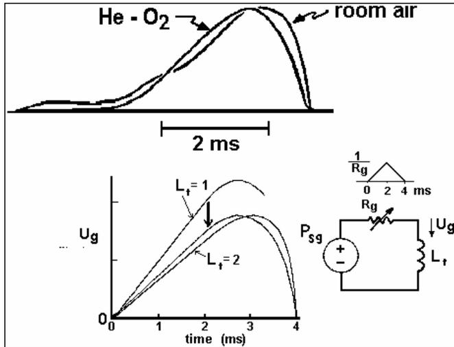
In this slide, the helium-oxygen results are compared with the airflow pulse waveforms obtained from the simple model for source-tract inertive interaction. For the model results, only two inertance values are shown and the amplitudes for the two values of inertance have been normalized to expedite visual comparisons. The similarities between the model result and the result from the lowering of inertance by breathing helium are apparent.
