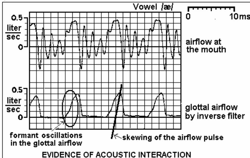
Next let us look at the acoustic interaction caused by the strong first formant energy just above the glottis. In the example in the figure, there is an oscillation at the frequency of the first formant in the glottal airflow pulse. This is not an error in inverse filtering – the oscillation represents formant energy passing from the supraglottal vocal tract into the trachea as the vocal folds separate. Note that the oscillations in the airflow at the mouth decrease more rapidly as a result.
