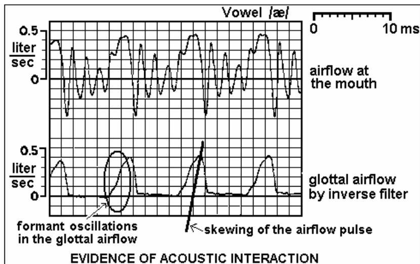
Acoustic interaction refers to the acoustic properties of the vocal tract affecting the airflow at the glottis (but not necessarily the vibratory pattern of the vocal folds). It was clear from the earliest inverse filter results, going back over 40 years, that at least two types of interaction between the vocal tract acoustics and the airflow at the glottis were present, as indicated in the slide.
