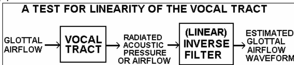
If a linear inverse filter can be derived that yields an accurate estimate of the glottal airflow waveform, then the vocal tract can be considered a linear system.
