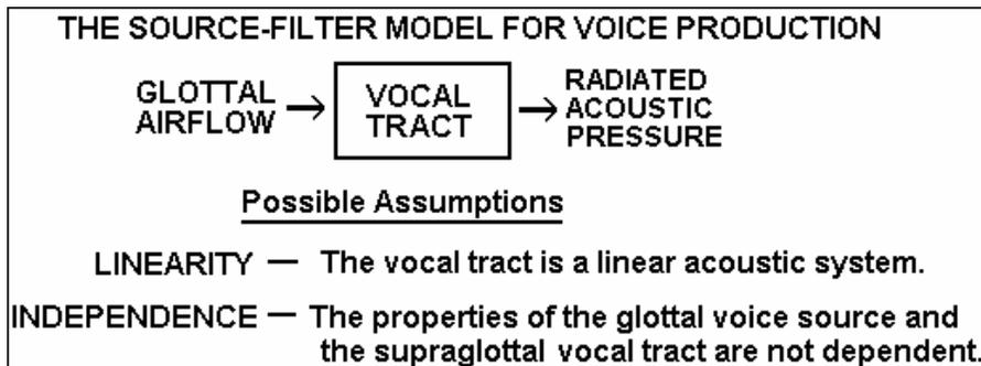
In the source-filter model, linearity and independence are separate assumptions, and either can hold without the other. Note that it is the vocal tract as an acoustic system that is assumed linear in the source-filter model, and not the glottis as a valve for airflow. In the simplest model, both properties are assumed to hold. This model is useful for pedagogical purposes, some speech synthesis applications and, more generally, as a first approximation for non-breathy voiced speech.
