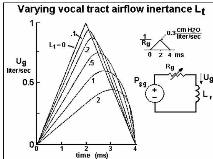
A few years later we found a solution to the differential equation for the simple model in Slide 7 for interaction with vocal tract inertance that enabled us to plot the airflow pulse waveform for varying values of vocal tract inertance, assuming a symmetrical triangular variation in glottal flow
