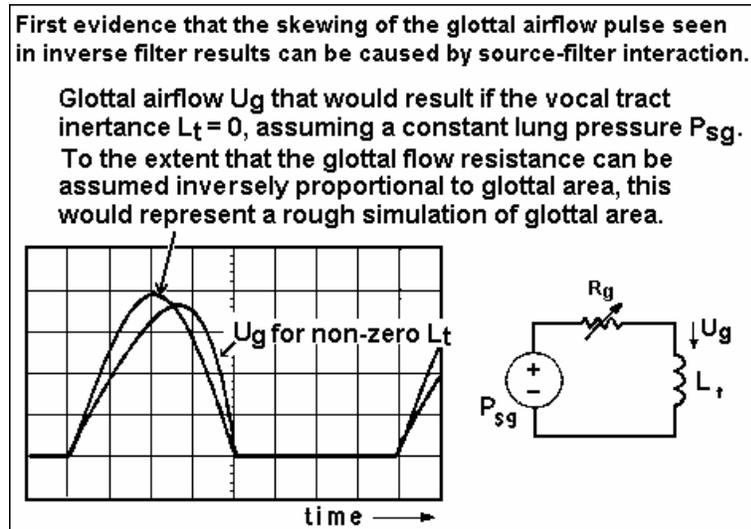
The mechanism causing the skewing of the glottal airflow pulse, especially pronounced in strong voices, was first described in conjunction with this figure taken from an electrical simulation reported in article in the *Journal of the Acoustical Society* in 1977. The element  $L_t$  simulated the inertance of the air in the vocal tract (and possibly the glottis and the trachea near the glottis).
