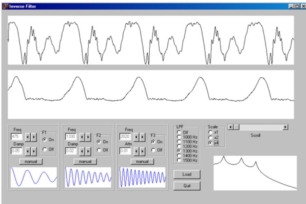
Figure 5. Screen layout for a digital inverse filter having all the functionality of a manual filter.
