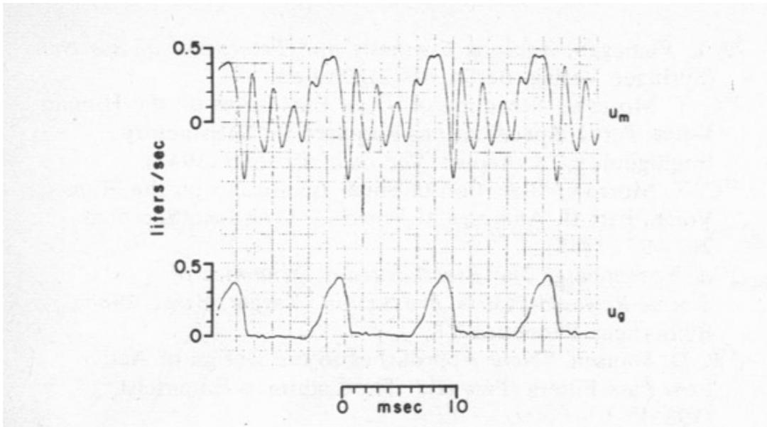
**Figure 2. Waveform from a CV mask for a held vowel /a/ by an adult male speaker, for which the value of F1 was much higher than F0, showing the strong oscillation at the frequency of F1 during the glottal closed phase [above], and the glottal airflow obtained by inverse filtering the waveform from the CV mask [below]. [from Rothenberg, 1973]**
