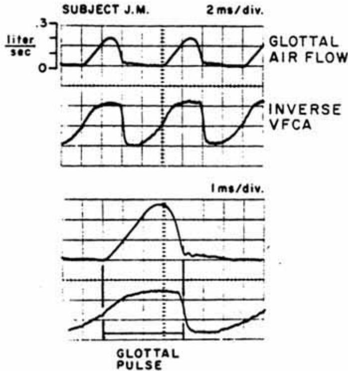
**Figure 3. Simultaneous glottal air flow waveform obtained by inverse filtering and electroglottograph waveform, showing the mutual corroboration of both the open glottis interval (the "glottal pulse") and period of glottal closure. [from Rothenberg, 1979]**
