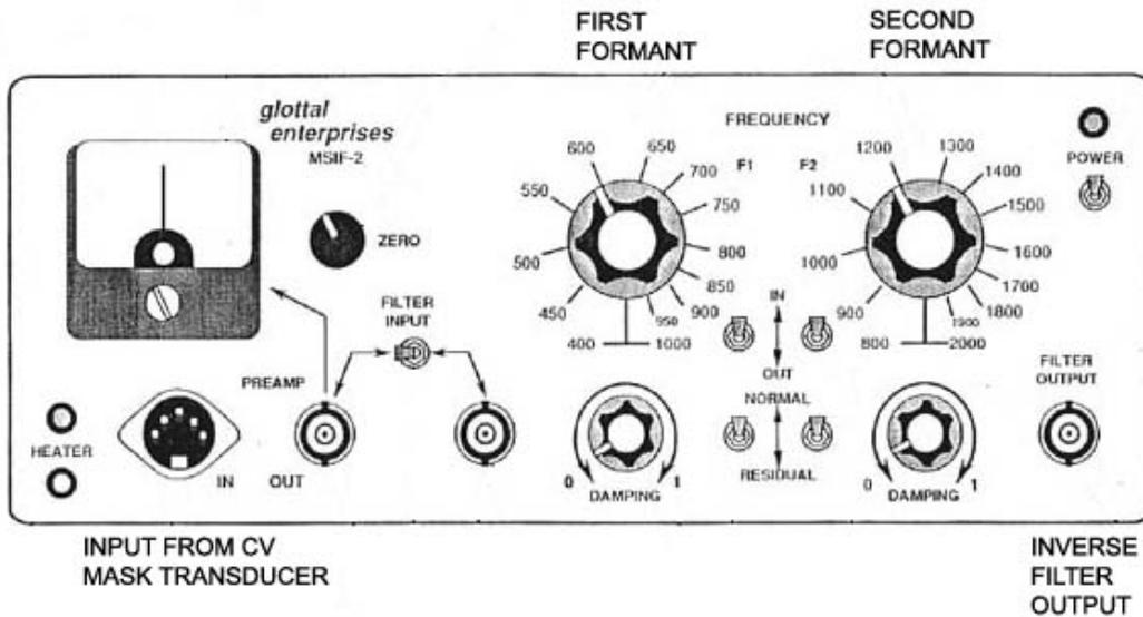
**Figure 1. A two-formant hardware inverse filter.**
