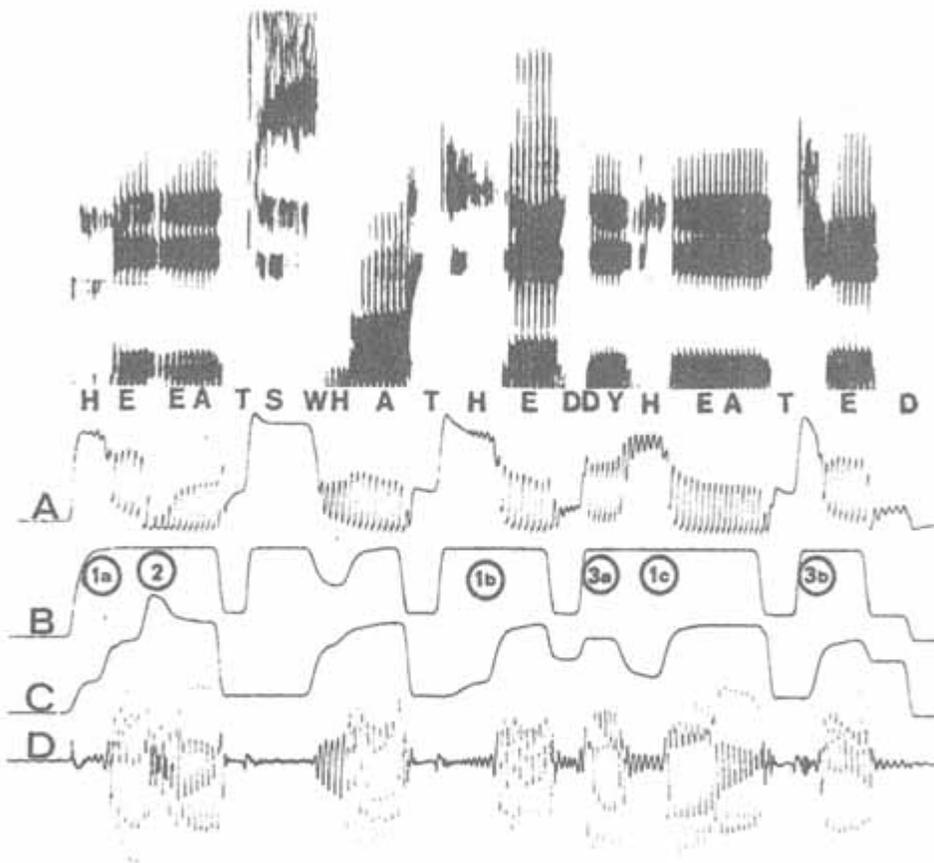
Fig. 6. The utterance "He eats what Hedy heated" synthesized with the aid of the new voice source. Curve A: simulated glottal airflow. B: the "loudness" control L. C: the "tightness" control T. D: audio output from the synthesizer. Figures in circles refer to interesting parts discussed in the text.
