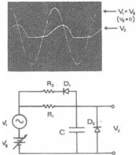
Fig. 1. Basic circuit for the voice source and illustrative waveforms.
