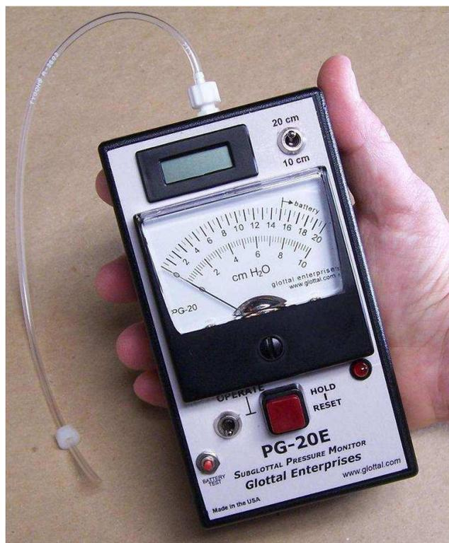
**FIGURE 16.** Device for providing a real-time approximation to subglottal pressure during speech.
