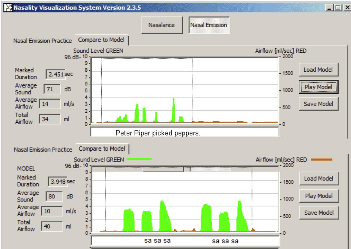
**FIGURE 3.** Examples showing that there is no appreciable nasal emission during pressure consonants in normal speech.
