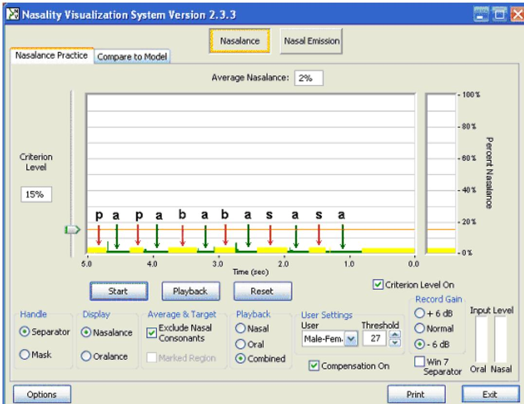
**FIGURE 10.** Vowels between the pressure consonants /p/, /b/, and /s/, showing a minimum of nasalance (2% average for the vowel /a/). The yellow bars indicate that the voiced energy in the oral and nasal channels at that instant was below a preset threshold and no nasalance measurement was possible. Thus these yellow bars mark the /p/ /b/ and /s/ consonants and a period of silence after the final vowel.
