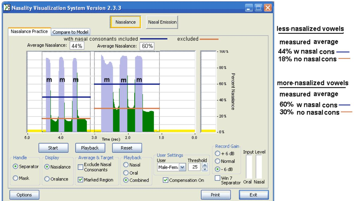
**FIGURE 8. Minimally nasalized and highly nasalized vowels in a nasal consonant context, testing the effect of excluding the nasal consonants in the averaging.**
