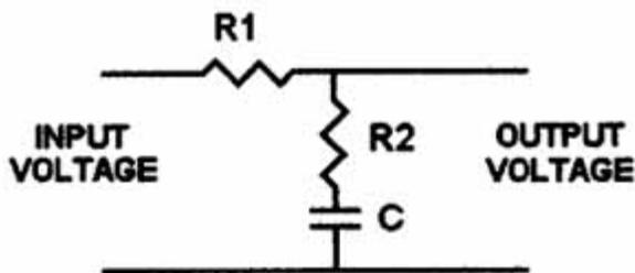
**FIGURE 3.** Simple compensation circuit for reducing the low-frequency phase distortion caused by high-pass filtering.
