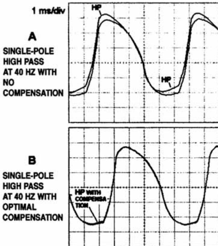
**FIGURE 4.** Effect of the compensator of Figure 3 in reducing the phase distortion present in the high-pass filtered EGG waveform of Figure 2B.
