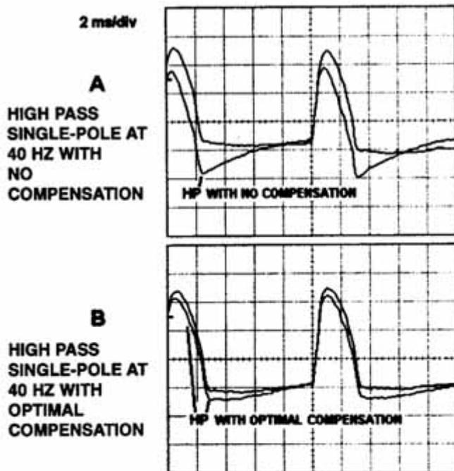
**FIGURE 6.** Optimal compensation of an EGG waveform of the type for which the distortion caused by high-pass filtering is greatest, namely at a low  $F_0$  (approximately 95 Hz) and exhibiting a low closed quotient (approximately 0.30).
