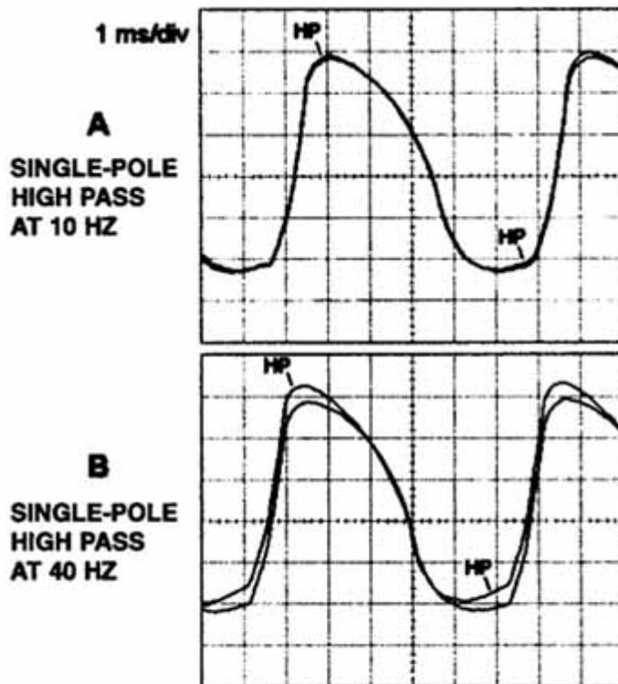
**FIGURE 2.** Effect on a typical EGG (vocal fold contact area) waveform of single-pole high-pass filters having  $-3$  dB frequencies of 10 and 40 Hz.
