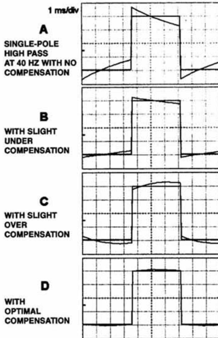
**FIGURE 5.** Compensated high-pass filtered waveforms showing the effect of varying the compensator parameters about a value subjectively judged to be optimal.
