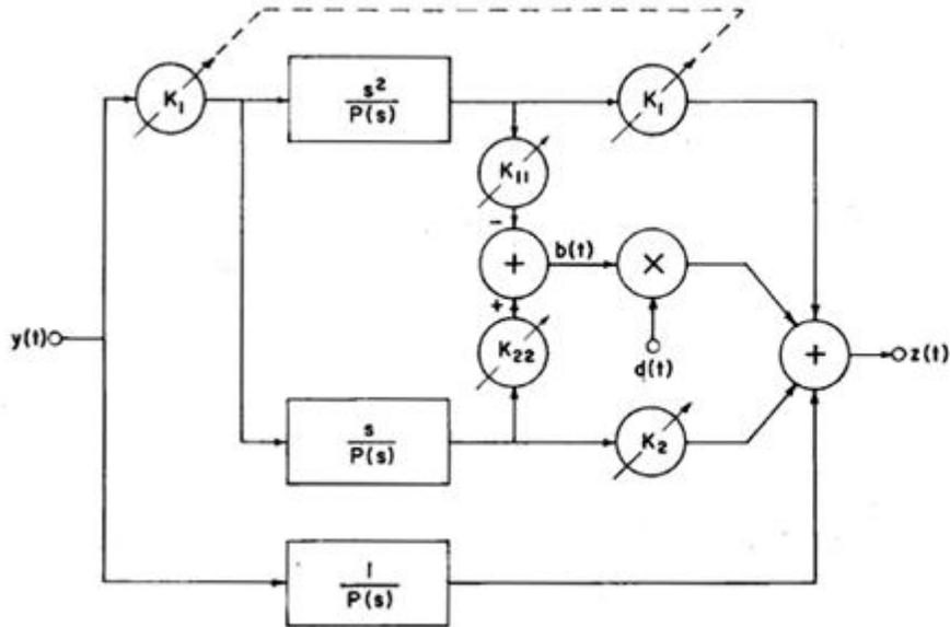
FIG. 6. Time-varying inverse filter.
