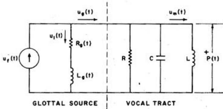
FIG. 4. Simplified electrical network model of glottal source/vocal tract system.
