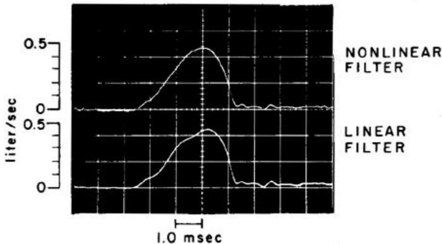
FIG. 10. Nonlinear inverse filtering of a spoken vowel [æ]. The top trace shows the output of the time-varying nonlinear inverse filter. The bottom trace shows the output of the time-invariant inverse filter.
