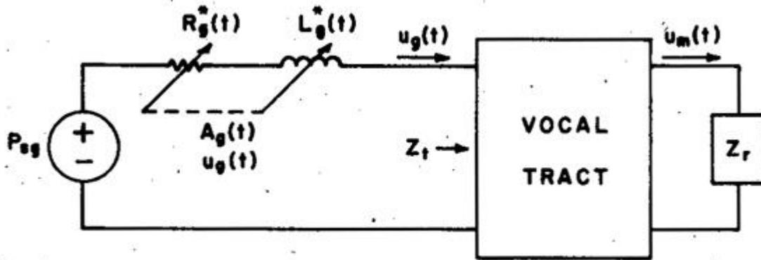
FIG. 1. Model for the glottal-supraglottal system.
