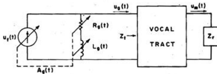
FIG. 3. Norton equivalent model for the glottal source during voicing.
