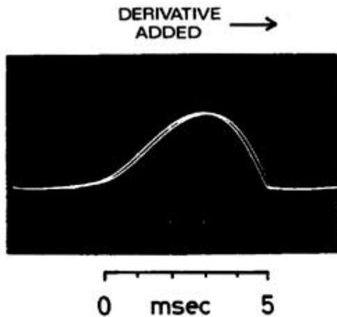
FIG. 12. Effect on a simulated glottal airflow pulse  $u_t$  of adding a term  $-K(du_t/dt)$  to simulate the air displaced by the motions of the vocal folds.
