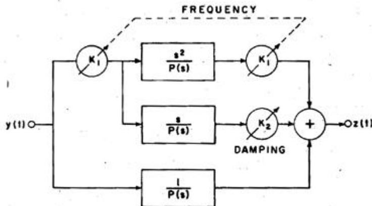
FIG. 5. Time-invariant inverse filter for a single formant.
