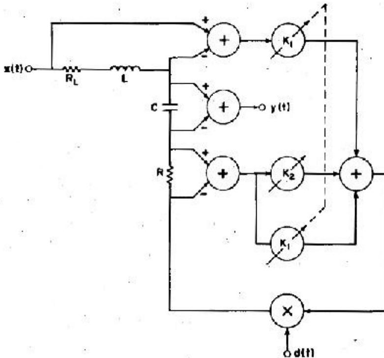
FIG. 7. Time-varying filter.
