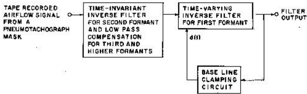
FIG. 9. System for nonlinear inverse filtering of real speech.
