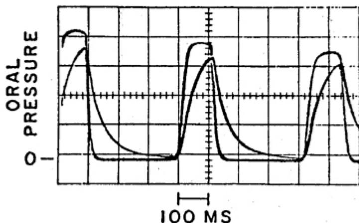
**FIGURE 1.** Intraoral pressure during contiguous repetitions of the syllable /pa/ as measured by two transducer systems having different response times.
