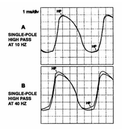
FIGURE 2. Effect on a typical EGG (vocal fold contact area) waveform of single-pole high-pass filters having -3 dB frequencies of 10 and 40 Hz.
