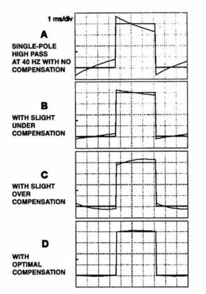
FIGURE 5. Compensated high-pass filtered waveforms showing the effect of varying the compensator parameters about a value subjectively judged to be optimal.
