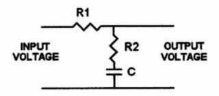
FIGURE 3. Simple compensation circuit for reducing the lowfrequency phase distortion caused by high-pass filtering.
