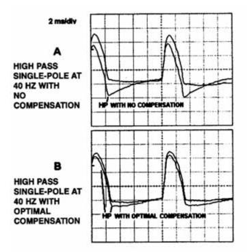
**FIGURE 6.** Optimal compensation of an EGG waveform of the type for which the distortion caused by high-pass filtering is greatest, namely at a low  $F_0$  (approximately 95 Hz) and exhibiting a low closed quotient (approximately 0.30).
