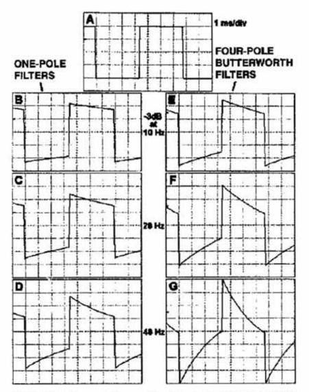
FIGURE 1. Changes in the waveform of a square pulse caused by the low-frequency phase distortion introduced by a high-pass filter.
