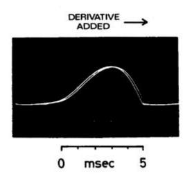
FIG. 12. Effect on a simulated glottal airflow pulse  $u_t$  of adding a term  $-K(du_t/dt)$  to simulate the air displaced by the motions of the vocal folds.
