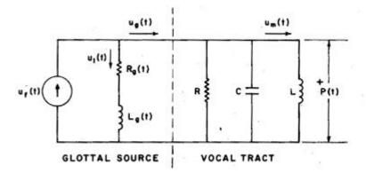
FIG. 4. Simplified electrical network model of glottal source/vocal tract system.
