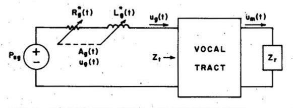
FIG. 1. Model for the glottal-supraglottal system.
