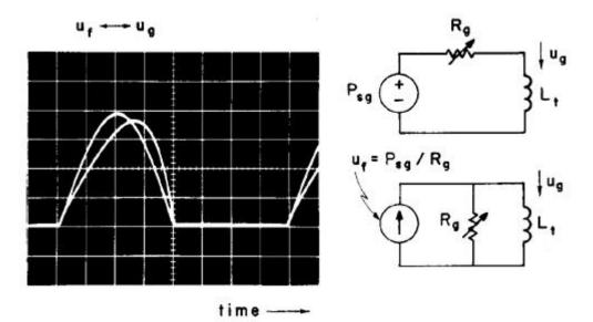
FIG. 11. Change in the glottal volume velocity waveform caused by the interaction of a time varying glottal resistance and an inertive supraglottal vocal tract loading. At the right are the Thevenin and Norton equivalent models for the system used in the simulation.
