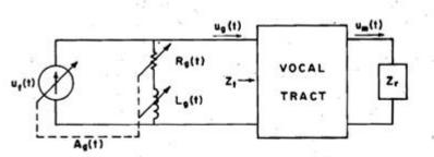
FIG. 3. Norton equivalent model for the glottal source during voicing.
