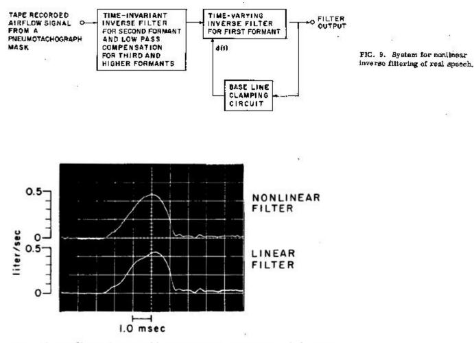
FIG. 10. Nonlinear inverse filtering of a spoken vowel [x]. The top trace shows the output of the time-varying nonlinear inverse filter. The bottom trace shows the output of the time-invariant inverse filter.
