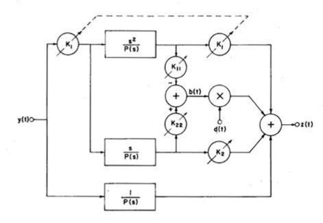
FIG. 6. Time-varying inverse filter.
