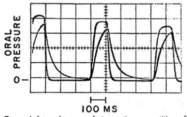
FIGURE 1. Intraoral pressure during contiguous repetitions of the syllable /pa/ as measured by two transducer systems having different response times.
