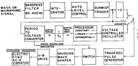
FIG. 1. System used for converting voice fundamental frequency to vibro tile pulse frequency.
